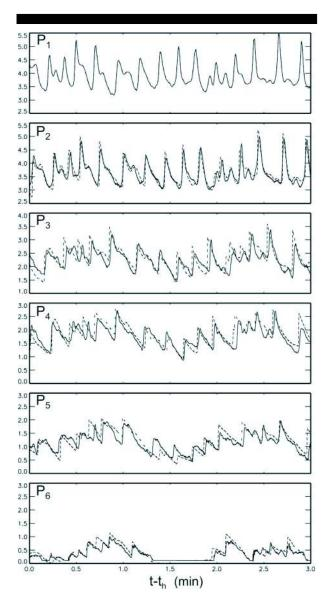
Figure 4. Comparison between observed (solid line) and predicted (dashed line) time series of water depth at sensors P1-6;  $t=t_{h}$ .
