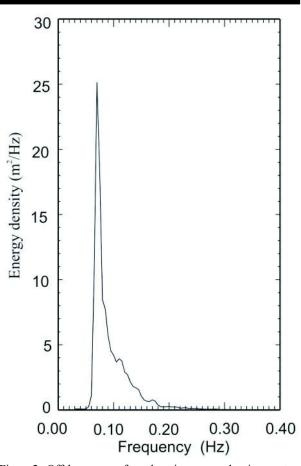
Figure 2. Offshore sea surface elevation energy density spectra measured in 56 m water depth on October  $18^{th} 2001$  at high tide  $(t=t_{h})$ .
