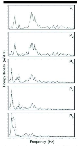
Figure 5. Comparison between observed (solid line) and predicted (dashed line) sea surface elevation density spectra at sensors P1-5;  $t=t_{h}$ .
