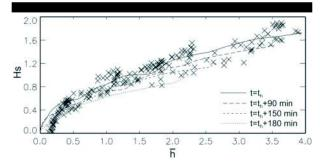
Figure 7. Observed (X) and predicted (line) significant wave height versus mean water depth. Experimental data correspond to the whole data set (te[t<sub>h</sub>-127 min,  $t_h$ +203 min]).
