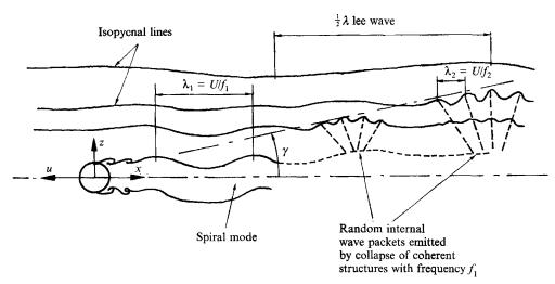
FIGURE 12. Schematic representation of internal waves emitted by the turbulent wake.
