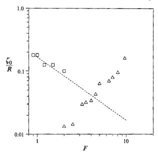
FIGURE 7. Internal wave amplitude  $\zeta_0$ , normalized by R, as a function of Froude number, measured at 3R above the centre of the sphere and 80R downstream. Re(1) = 2614; ----, linear theory of lee wave;  $\Box$ , lee wave amplitude;  $\triangle$ , random wave amplitude.
