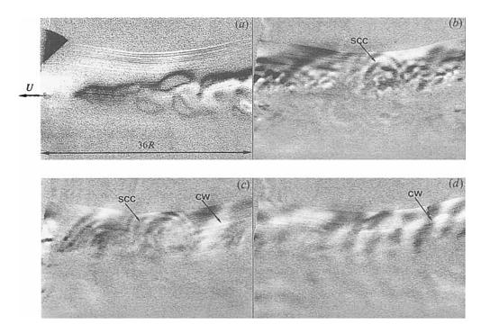
FIGURE 9. Visualization of the random-coherent waves in a horizontal plane, |z| = 3R (R = 3.6 cm) below the centre of the sphere, for F = 5 and Re(1) = 2614. (a) Nt = 0; (b) Nt = 35.1; (c) Nt = 52.6; (d) Nt = 87.7. CW, coherent wave; SCC, semicircular concentric wave.
