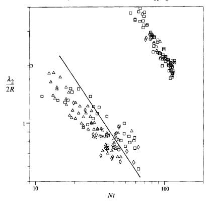
FIGURE 8. Wavelength of the random waves, normalized by 2R, as a function of Nt. Re(1) = 2614;  $\triangle$ ,  $F = 10/\pi$ ;  $\diamondsuit$ , F = 4;  $\square$ , F = 5. The solid line shows equation (12).
