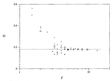
FIGURE 13. Strouhal number as a function of the Froude number.  $\triangle$ ,  $St_w$  measured outside the wake at x/R = 80; \*, Strouhal number of the wake instability measured inside the wake at Nt < 2.5.
