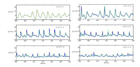
Figure 4. Time windows for measured and computed free surface at different spatial locations. (-) measured, (--) computed with CIEN model, and (-.-) computed with KENN model.
