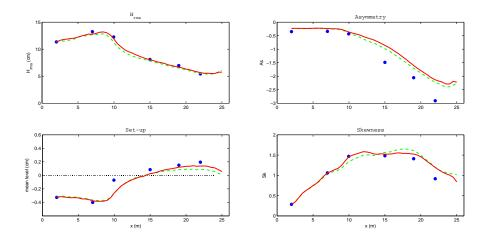
Figure 5. Wave properties. (•) measured, (--) computed with CIEN model, and (-) computed with KENN model.
