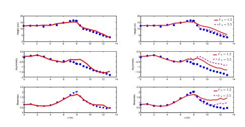
Figure 2. Comparison between measured (•) and computed (-, --) wave properties for Ting and Kirby (1994) experiment. Left panel: CIEN breaking model. Right panel: KENN breaking model.
