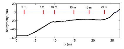
Figure 3. Bottom profile and wave gauge locations for the random wave experiment.
